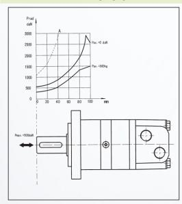
The output shaft runs in tapered bearings that permit high axial and radial forces, Curve "A" shows max radial shaft load, Any shaft loads exceeding the values quoted in the curve will involve a risk of breakage, The two other curves apply to a B10 bearing life of 3000 hours at 200 RPM.
