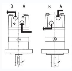
When facing shaft end of motor, shaft to rotate: Clockwise when port "A" is pressurized. Counter-clockwise port "B" is pressurized.
